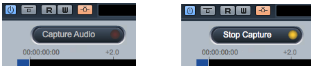
Figure 17 Selecting Capture Audio (left) after which the light in the button glows yellow and shows 'Stop Capture' (right)
