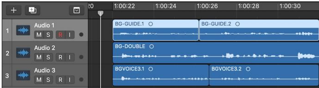
Figure 32. Selecting the Guide and Dub(s). In this example, the audio regions BG-Guide.1 and BG-Guide.2 could be selected to form the Guide. Likewise, BG-Voice3.1 and BG-Voice3.2 could be selected as one Dub and BG-Double as another.
