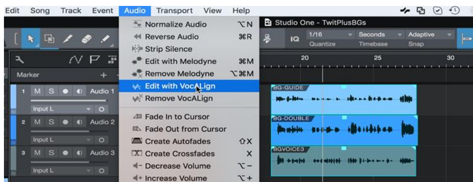
Figure 25 VocAlign Pro is added as an Event Fx using Edit with VocAlign in Studio One's Audio Menu
