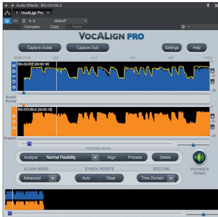
Figure 35 VocAlign Pro displays the energy profiles of the Guide (blue) and Dub (orange). The yellow trace shows the energy profile of the Aligned Dub.
